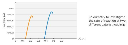
The calorimetry combined with mechanistic understanding pointed to a problem with the transmetallation of the aryl boronic ester in the reaction. A change of base from potassium carbonate to sodium hydroxide resulted in a complete clean conversion of both starting materials to afford the desired high purity product. The new cleaner reaction permitted a simple isolation by crystallisation. The whole study took approximately 1 week.
